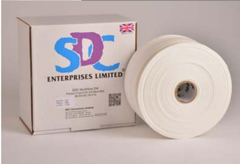
There are no weaving oils used in the manufacture of SDCE Multifibre, thus preventing the need for subsequent wet processing and heat treatments which are a potential source of inconsistency and contamination. This gives a dimensionally stable product that does not suffer slippage/separation of warp yarns or fraying during test procedures.
