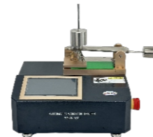
Scratch Tester Sample size: 100 x 150mm Sample thickness: MAX 1.6mm Test coating thickness: 0.3mm
