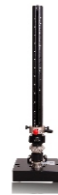
Impact Tester Weight of indenter: 1kg Tube height: 100cm Compliant with standards: ISO6272, BS3900, DIN55669
