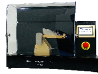
Automatic Cylindrical Bend Tester Bending times: 1~99999 times Speed: 10~60rpm Sample thickness: 0.3-1mm
